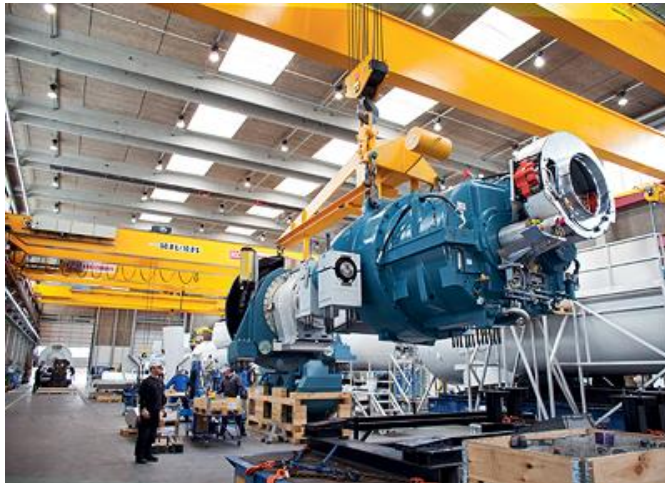
Assembled 2.3-MW nacelle (Siemens website)
